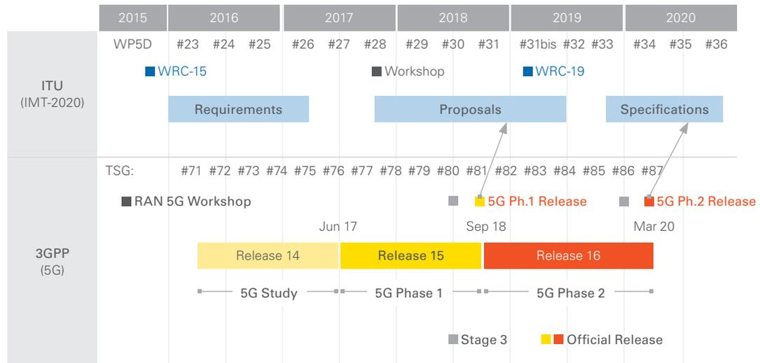
Figure 1. 5G Timelines From ITU and 3GPP. Source: Netmanias
