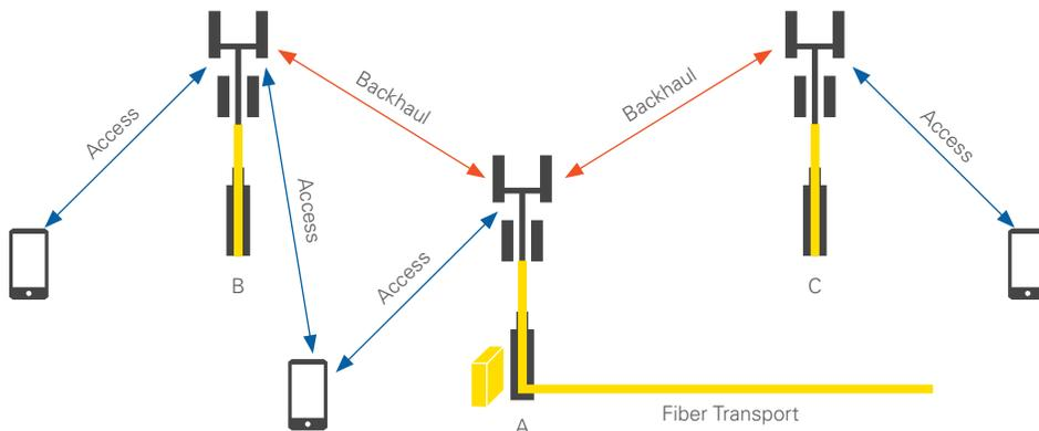
Figure 4. Illustration of IAB. Source: RP-170831
