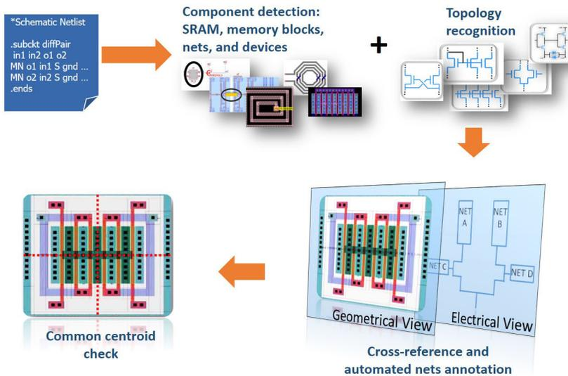
Figure 2: The Calibre PERC platform provides the infrastructure and automation required for context-aware checking, such as common centroid assessment.
