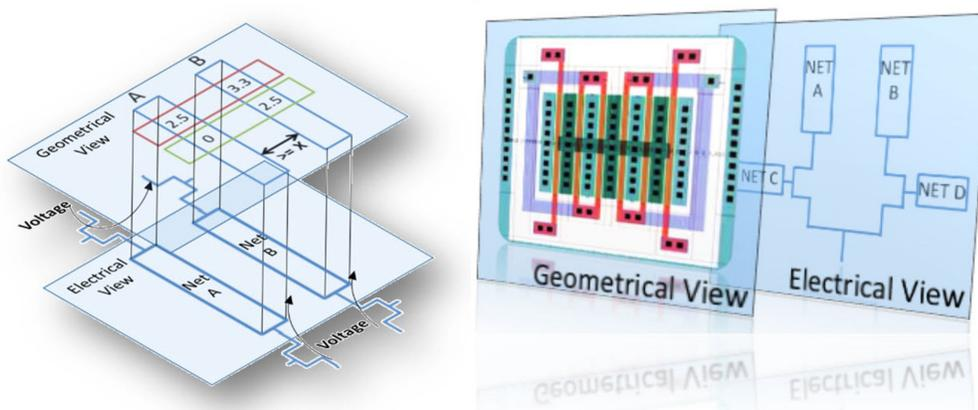
Figure 1: Context-aware checks combine geometrical and electrical aspects to determine design rule compliance.
