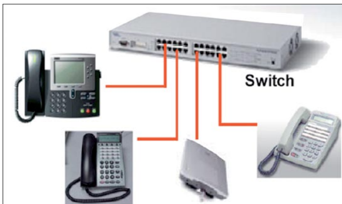
Figure 1a: Shown is an endpoint PoE implementation, with the end application hooked up to the switch.
