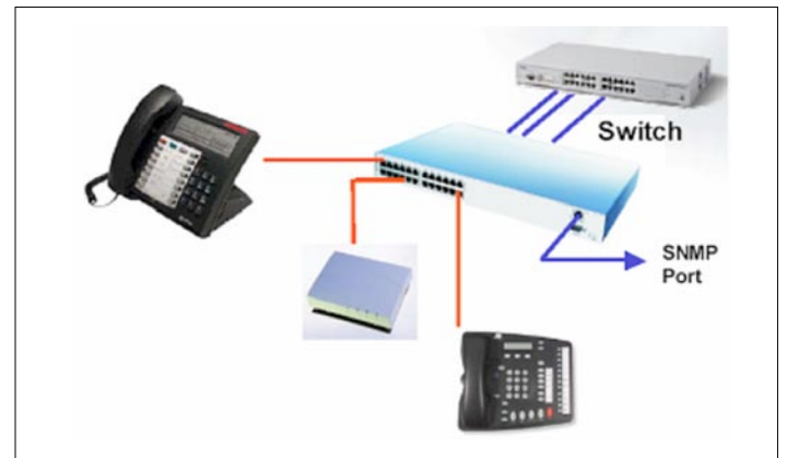
Figure 1b: Shown is the mid-span implementation of PoE, wherein the power is inserted to the network.
